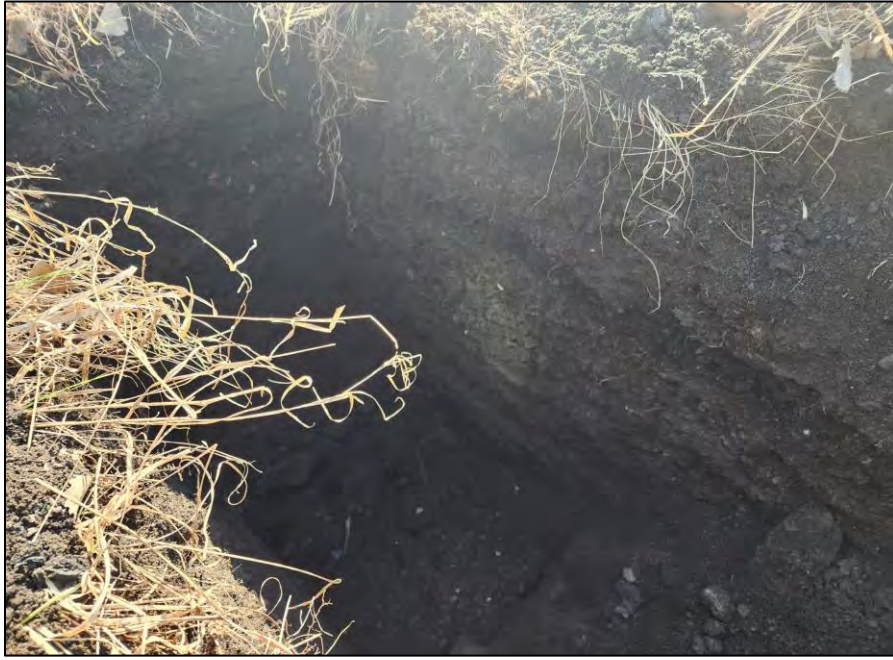
Photo 3. March 13, 2025. Test trench 2 showing apparent CCR layers.
