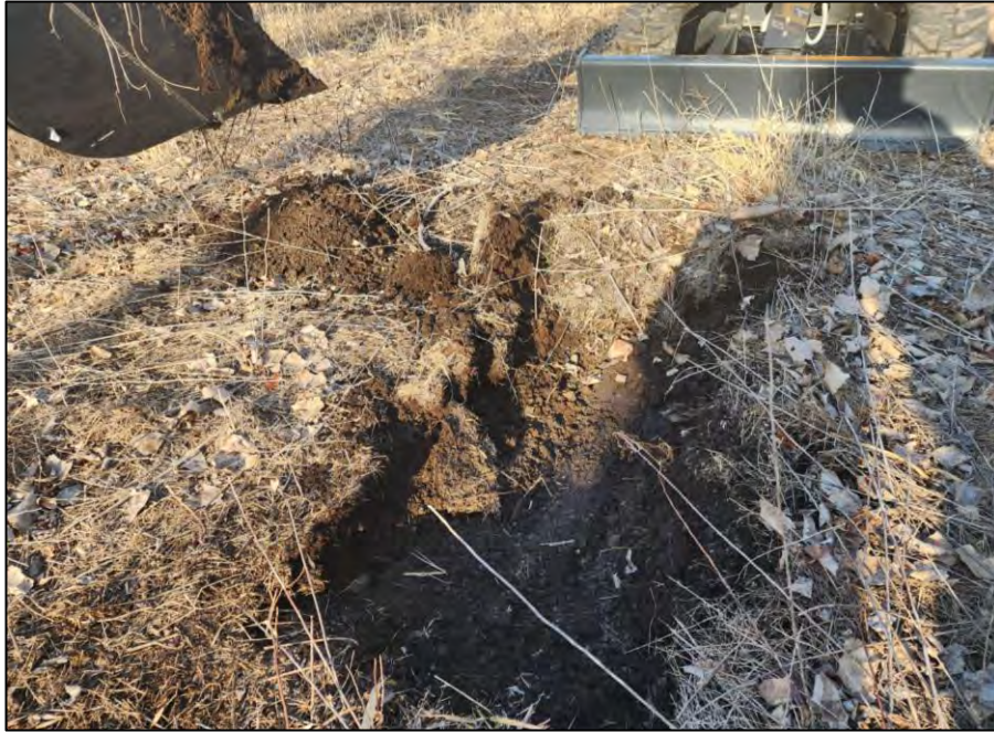
Photo 1. March 13, 2025. Test trench 1 showing initial surface conditions and shallow CCR.
